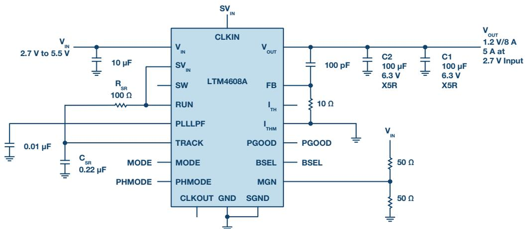
Figure 5. LTM4608A with spread spectrum enabled.
