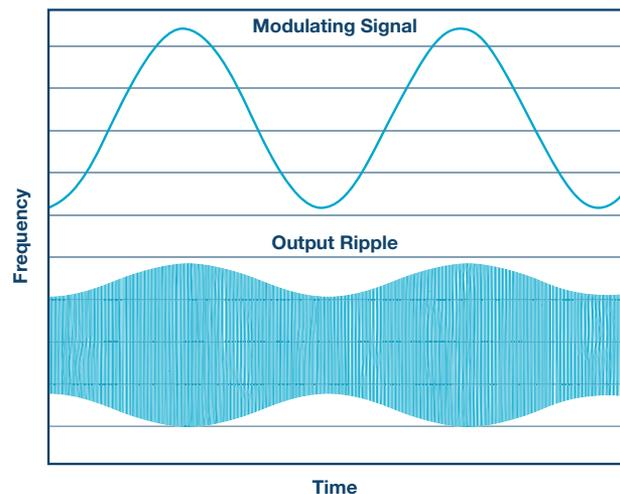
Figure 1. Illustration of switching regulator ripple due to sinusoidal frequency modulation of the clock.
