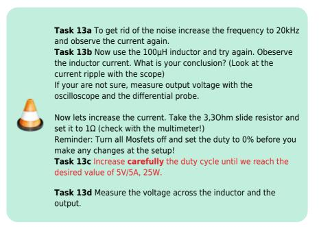
Okay, it's still not ideal. If you want, you can increase the inductance value, adjust the frequency (max. 40 kHz), and observe whether you can further reduce the ripple current.
