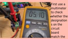
measured polarity **before connecting the capacitor**. It might be possible that the incuctor is in the return current path by mistake.
