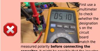
**capacitor**. It might be possible that the incuctor is in the return current path by mistake.
