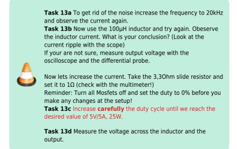
Okay, it's still not ideal. If you want, you can increase the inductance value, adjust the frequency (max. 40 kHz), and observe whether you can further reduce the ripple current.
