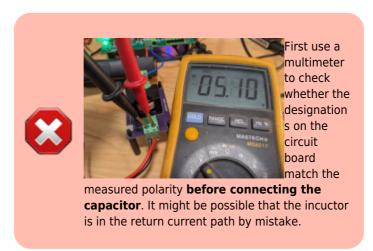
In the next task, we will try to smooth the output voltage and reduce the output current ripple using capacitors. For a higher resolution of the ripple, you can filter out the average value of a signal by switching to **AC coupling** on the oscilloscope. As a result, a capacitor is connected in series with the signal at the oscilloscope input, blocking the average value. It is now possible to fully zoom out the remaining ripple and determine it using the cursor.
