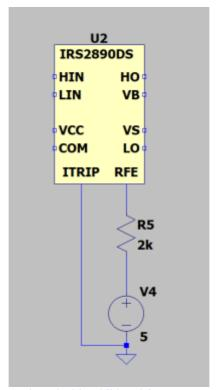
Gate drivers are often equipped with additional features. Our driver can detect overcurrents and if necessary, will turn off all MOSFETs for safety. Since overcurrents in a simulation tool will not damage your PC or notebook, you can ignore this feature in the simulation. Pull up the RFE output and connect ITRIP to ground.
