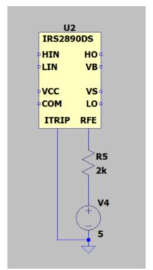
Gate drivers are often equipped with additional features. Our driver can detect overcurrents and if necessary, will turn off all MOSFETs for safety. Since overcurrents in a simulation tool will not damage your PC or notebook, you can ignore this feature in the simulation. Pull up the RFE output and connect ITRIP to ground.
