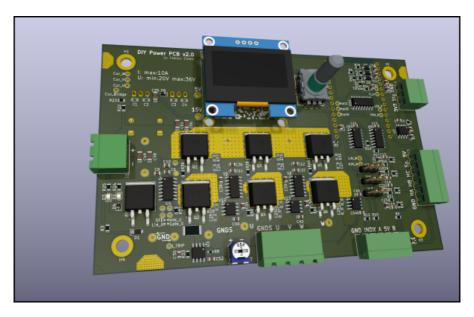
The PCB was originally not only developed for the power electronics lecture but also to drive different motor applications. Therefore, the PCB contains more features than are necessary for your measurements.
