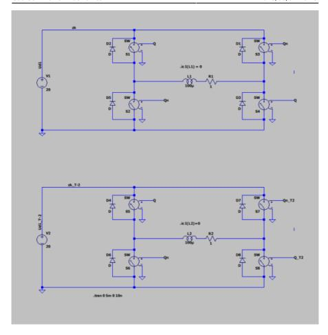
When using labels to assign node names in your schematic, all nodes with the same label are electrically connected. This simplifies schematic design but also requires careful attention. Incorrect or careless use of labels can lead to unintended connections and, in the worst case, short circuits. Always double-check your labeling to ensure that only intended nodes share the same potential.
