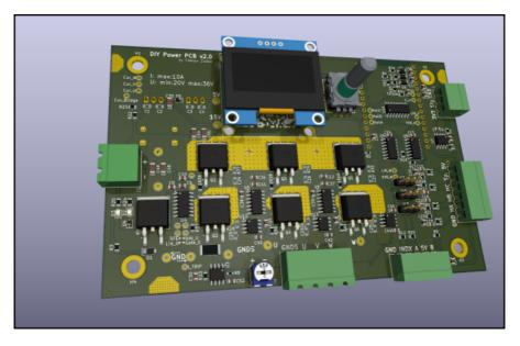
The PCB was originally not only developed for the power electronics lecture but also to drive different motor applications. Therefore, the PCB contains more features than are necessary for your measurements. Schematic and PCB files see: DIYPowerPCB
