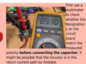
In the next task, we will try to smooth the output voltage and reduce the output current ripple using capacitors. For a higher resolution of the ripple, you can filter out the average value of a signal by switching to **AC coupling** on the oscilloscope. As a result, a capacitor is connected in series with the signal at the oscilloscope input, blocking the average value. It is now possible to fully zoom out the remaining ripple and determine it using the cursor.
