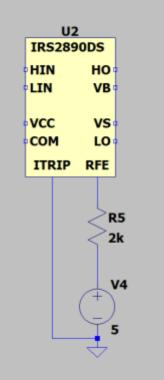
Gate drivers are often equipped with additional features. Our driver can detect overcurrents and if necessary, will turn off all MOSFETs for safety. Since overcurrents in a simulation tool will not damage your PC or notebook, you can ignore this feature in the simulation. Pull up the RFE output and connect ITRIP to ground.
