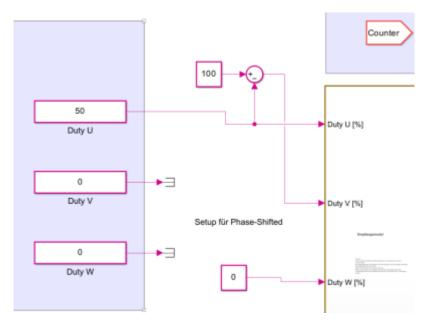
Additionally, using the microcontroller in combination with Simulink, we have the capability to implement a phase shift between PWM signals. For our purposes, the two relevant configurations are 0° and 180° phase shift. As described earlier, the mathematical trick used to compute the duty cycle for phase V by inverting the
