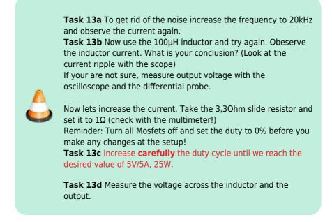
Okay, it's still not ideal. If you want, you can increase the inductance value, adjust the frequency (max. 40 kHz), and observe whether you can further reduce the ripple current.
