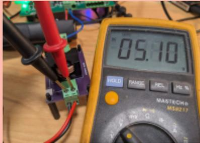
First use a multimeter to check whether the designations on the circuit board match the measured
