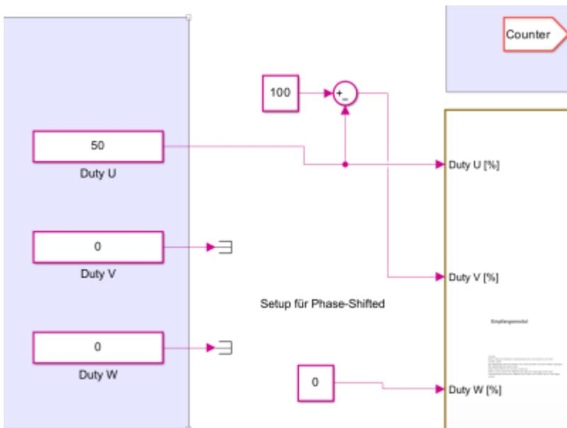
Additionally, using the microcontroller in combination with Simulink, we have the capability to implement a phase shift between PWM signals. For our purposes, the two relevant configurations are 0° and 180° phase shift. As described earlier, the mathematical trick used to compute the duty cycle for phase V by inverting the
