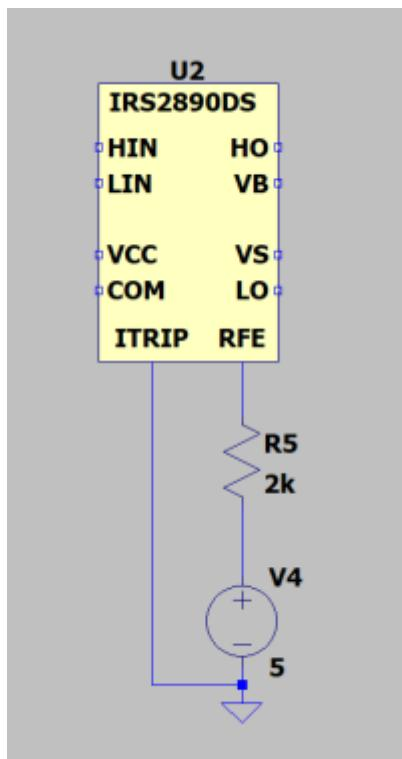
Gate drivers are often equipped with additional features. Our driver can detect overcurrents and if necessary, will turn off all MOSFETs for safety. Since overcurrents in a simulation tool will not damage your PC or notebook, you can ignore this feature in the simulation. Pull up the RFE output and connect ITRIP to ground.
