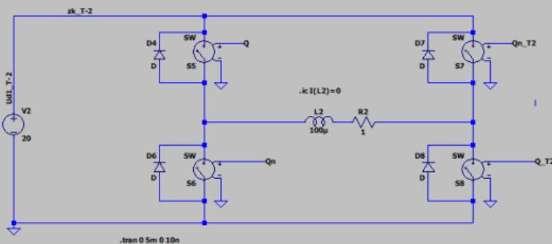
When using labels to assign node names in your schematic, all nodes with the same label are electrically connected. This simplifies schematic design but also requires careful attention. Incorrect or careless use of labels can lead to unintended connections and, in the worst case, short circuits. Always double-check your labeling to ensure that only intended nodes share the same potential.
