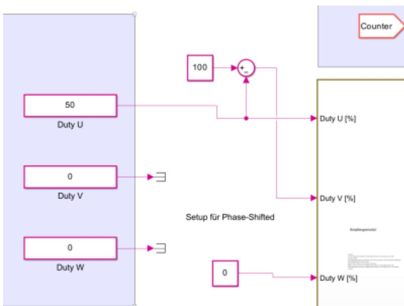
Additionally, using the microcontroller in combination with Simulink, we have the capability to implement a phase shift between PWM signals. For our purposes, the two relevant configurations are  $0^\circ$  and  $180^\circ$  phase shift. As described earlier, the mathematical trick used to compute the duty cycle for phase V by inverting the
