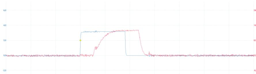
Take a screenshot of all four measurements for your report. Label the signals and the delay times. To work with stable signals on the oscilloscope, it is generally a good idea to use a PWM signal as the trigger source.
